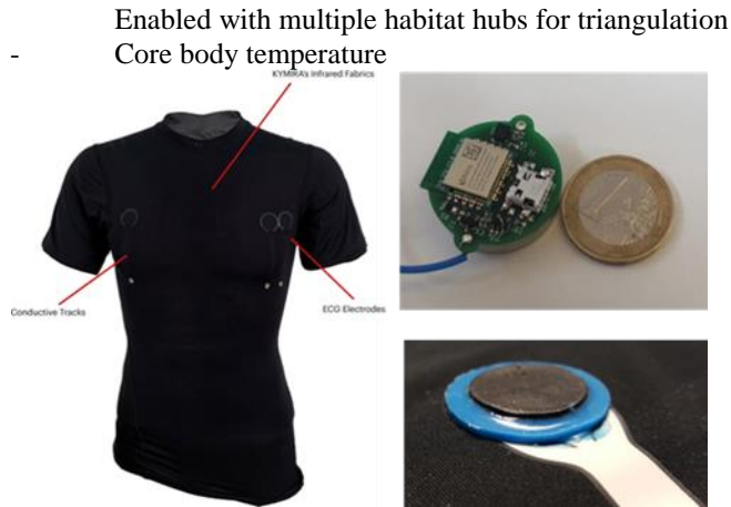
Fig .1 Kymira physiological measurement garment and sensors.
